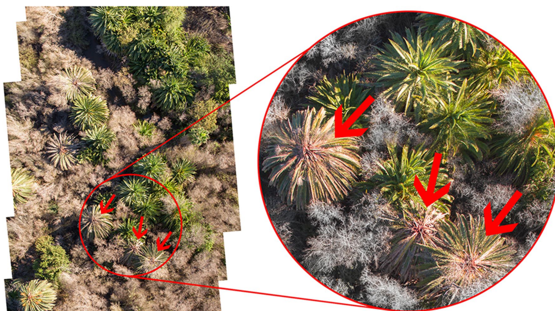
Fig. 7 Low-cost drones outfitted with high-resolution cameras can be programmed to fly specific routes over wilderness areas needing surveillance for palm weevil activity (red arrows). (Color figure online)
