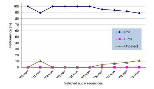
After processing each audio file, we compare the analysis results provided by our algorithm with the ones found at subjective tests, in order to obtain the values of the above defined performance metrics. Figure 8 shows the performance of our detection algorithm after processing the selected audio sequences. As it can be seen, there are no false positives, being the average detection rate around 96%.
