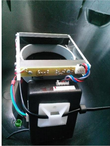
Figure 3. Detection device mounted on the funnel in the inside of the trap.
