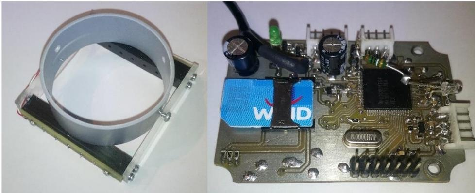
Figure 2. *Left*: optoelectronic sensor: A light gate guarding the lower part of the funnel. *Right*: microcontroller counting light interruptions, and message delivery.
