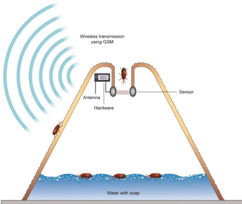
Figure 1. A typical plastic Picusan type trap with the optoelectronic detector embedded.
