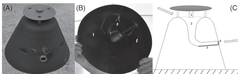
**Figure 1.** (A) Picusan trap with exit hole; (B) view from below of the infective trap design with inoculation tunnel; (C) trap sketch with components: (1) pheromone dispenser, (2) trap entrance with funnel, (3) infective tunnel, and (4) exit hole.
